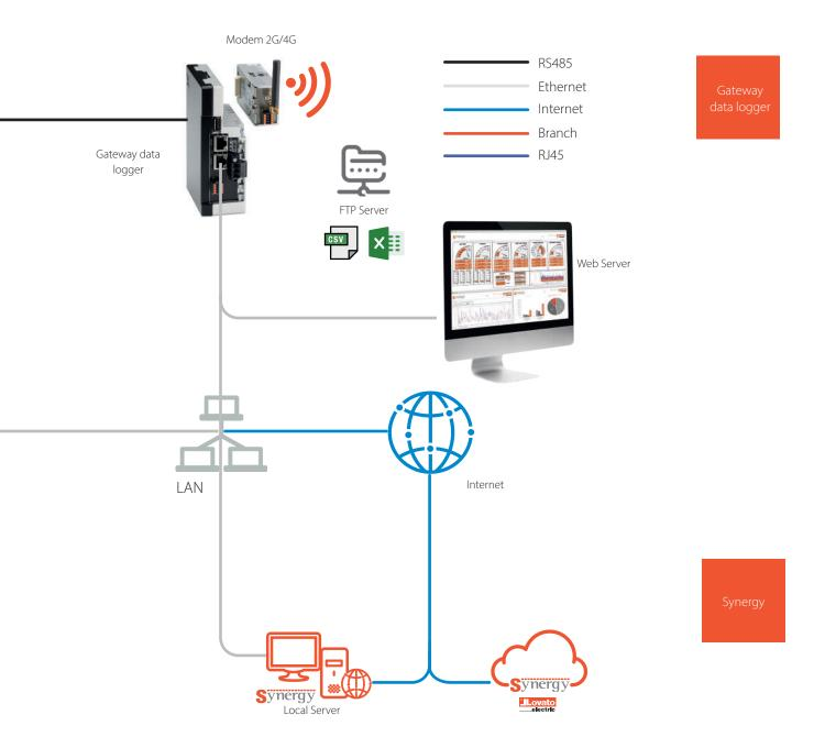
**Synergy** by LOVATO Electric is an energy monitoring and analysis system with a professional, flexible and integrated approach from an Industry 4.0 perspective. Thanks to the LOVATO Electric **measurement devices** equipped with a communication port and through the web-based supervision platform, it is possible to monitor real time measurements, consult graphics, receive alarms, export customized reports and carry out commands and settings.
