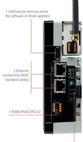
24VDC power supply (10...32VDC)
