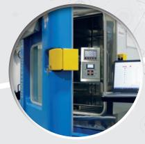
**ENVIRONMENTAL TESTS** Environmental tests: resistance to heat, damp heat and saline mist in climate chambers.
