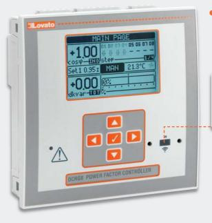
OPTICAL COMMUNICATION PORT By using CX 01 USB or CX 02 Wi-Fi point dongle, the optical port on the front allows to communicate with a PC, smartphone and tablet, to carry out programming, diagnotics and data download without removing power to the electric panel.
